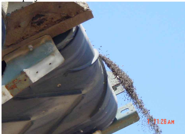
The fine particles shown coming off of the belt into the hopper are primarily lead shot.
