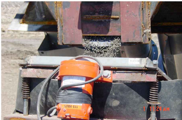
This photo shows shot dropping from the collecting hopper into a barrel.
