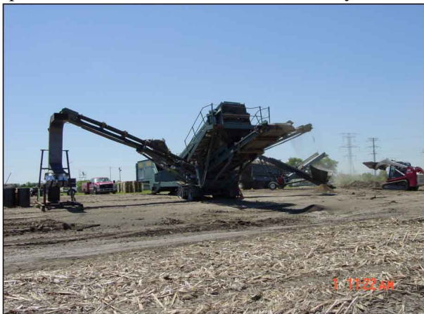
Loader on right feeds the system. Fine particles come off of the belt on the left.
